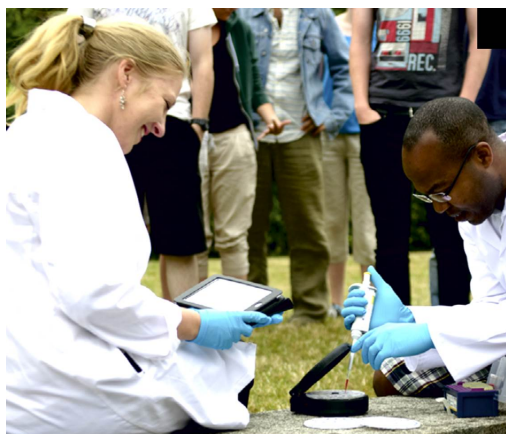
Figure 13. Testing of portable centrifugal microfluidic system for POC liver function testing in Nigeria. Reprinted from [117] with permission from Elsevier.
