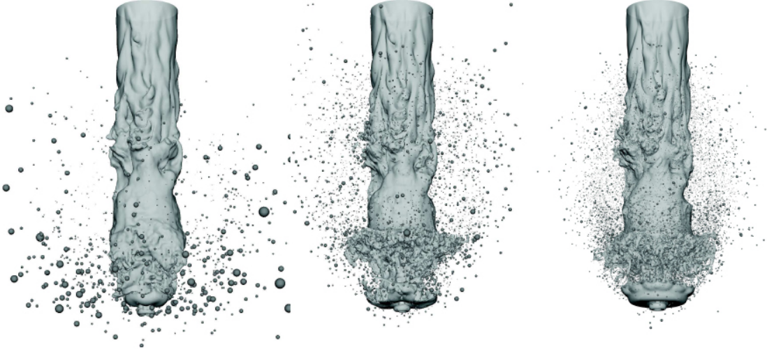
Figure 1.15: Impact of G-grid resolution at t = 4\mu s for constant flow solver resolution \Delta x = 1\ \mu m and \Delta x_G = 1.56\ \mu m (left), \Delta x_G = 0.78\ \mu m (center), and \Delta x_G = 0.39\ \mu m (right). Only the region close to the liquid core is shown [27].
