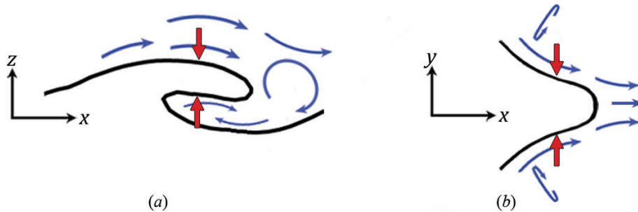
Figure 4.37: Schematic showing the lobe thinning in the normal direction in the LoHBrLiD process from a xz plane (a), and lobe thinning in the spanwise direction in the LoLiD process from a xy plane (b).
