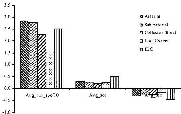
Fig. 4 Comparison of average running speed, acceleration and deceleration
