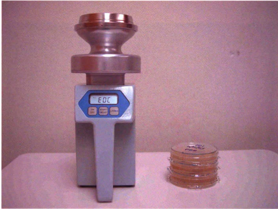
Figure 2. The air sampler, consisting of a rechargeable battery, timer, turbine, housing for culture plates, and removable sieve through which air is circulated to the culture plate.
