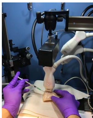
Figure 4.26 Experimental setup for ex vivo PA imaging.
