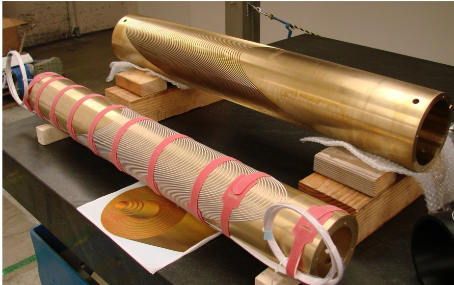
Figure 6.18: The 64 turn layer 1 and 2 mandrels for the NbTi test are shown. Layer 1 is wound with insulated NbTi cable.
