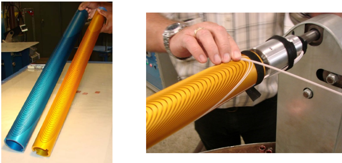
Figure 5.16: The anodized mandrels for layer 1 and layer 2 of CCT1 are shown. The mandrels were wound with conductor by hand with no additional applied tension.
