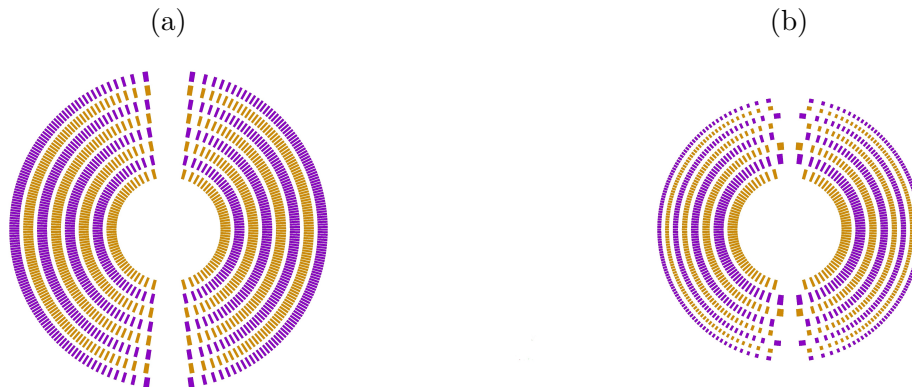
Figure 4.11: The ungraded (a) and graded (b) conductor cross sections are shown for the eight layer \text{Nb}_3\text{Sn} dipole design CCT2.
