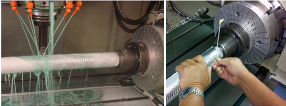
Figure 5.15: The CNC machining of an aluminum winding mandrel for CCT1 is shown.
