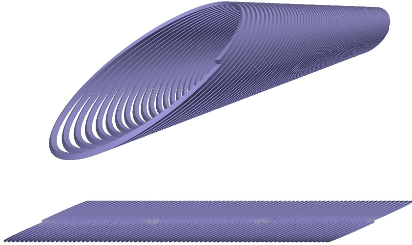
Figure 2.3: Two views of the conductor path for a CCT dipole layer are shown.
