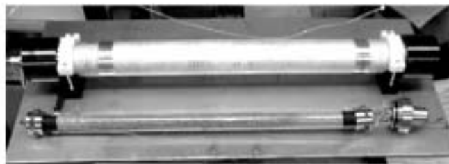
Figure 1. Photograph of experimental apparatus: aluminum confining vessel (background), and sand packing housed in a thin polycarbonate tube with stainless steel transducers containing acoustic source and receiver (foreground).
