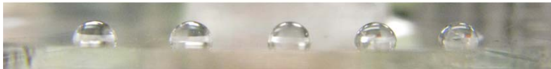
Figure 2-4. Using sessile-drop contact angles to compare silanization reactions and different surfaces. Above, the efficiency of triethylamine towards increasing the extent of silanization is shown by comparing contact angles of water droplets on the silanized glass surface. Below, representative contact angles for a series of different modified glass surfaces are shown.
