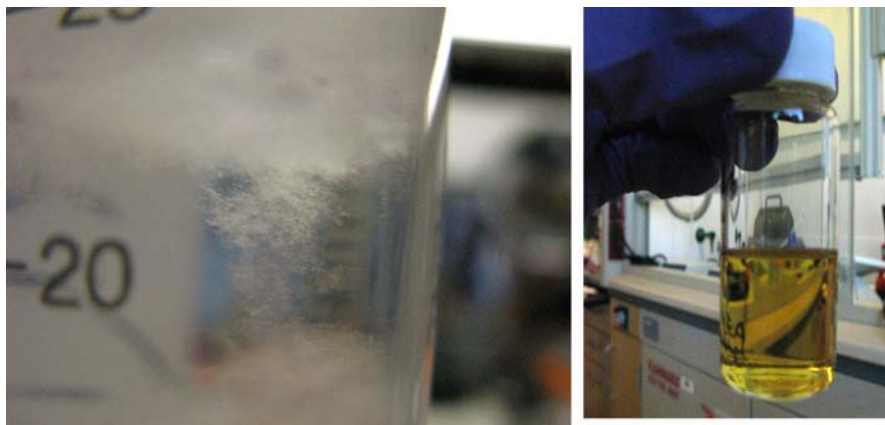
Figure 2-5. Failure modes when preparing silanization reactions. At left, a cottony precipitate forms when triethylamine and perfluorosilane are mixed in heptane or toluene. At right, color evolves when a reaction vessel is left alone for an hour.
