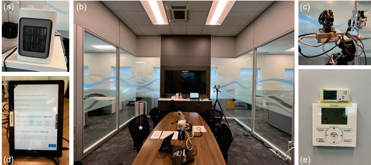
Figure 4. Demonstration configuration, showing photos of (a) the electric space heater used to simulate a summer heat load; (b) the conference room (about 4.3 m L × 4.3 m W × 3.7 m H), in which the subject’s chair is marked with an asterisk; (c) a close-up of the sensor-controller mounted on a tripod; (d) the survey tablet used to collect thermal sensation and comfort votes; and (e) a temperature/relative humidity logger mounted above the room’s conventional thermostat.
