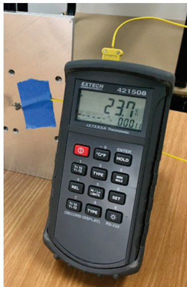
Figure 7. Image of the Extech 421508 Portable Thermometer w/ K-type thermocouple used at MoviTHERM.
