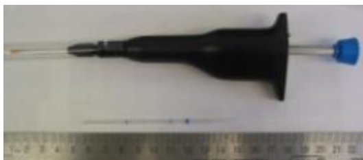
Figure A5. 100 uL Drummond Micro Pipetter (top) and tip (bottom) with ruler for scale.
