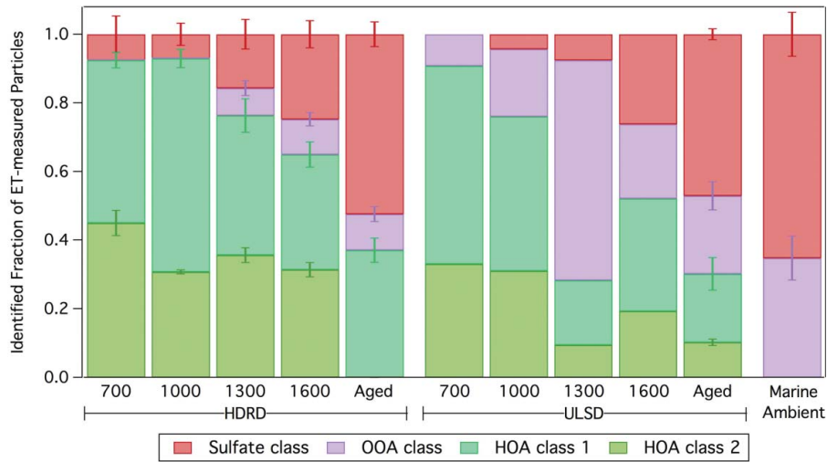
Figure 5. HR-ToF-AMS event trigger single-particle cluster analysis results for HDRD and ULSD emissions at 700, 1000, 1300, and 1600 rpm engine speeds as well as aged emissions, and marine background. The bars indicate the fraction of each identified particle class to the measured particle number. Four complete engine cycles (700–1600 rpm) were averaged for HDRD with whiskers showing the variability between cycles for each fraction. One complete engine cycle is shown for ULSD. The aged plume tests were divided into 1-h measurements (HDRD–4 h, ULSD–2 h). Marine ambient is the average of six separate 1-h marine background measurements. Individual measurement results are provided in Figure S4 in the SI. ET collection efficiency (CE) is likely particle-type-dependent. Therefore, the results are not CE-corrected.
