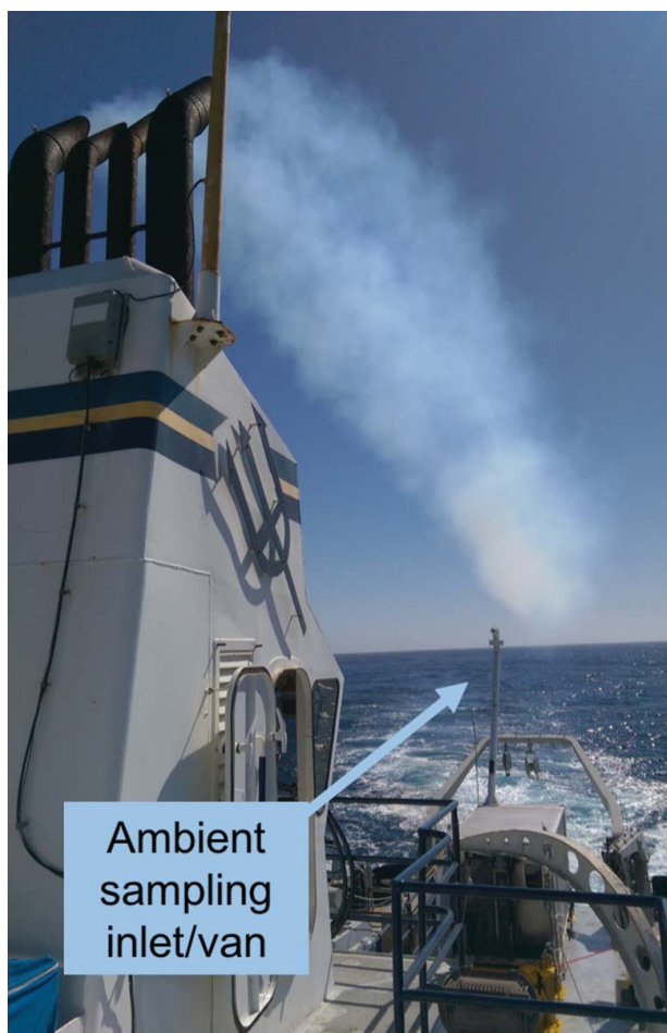
Figure 1. Picture of the exhaust stacks of the R/V Robert Gordon Sproull with the ambient sampling van secured to the aft deck.
