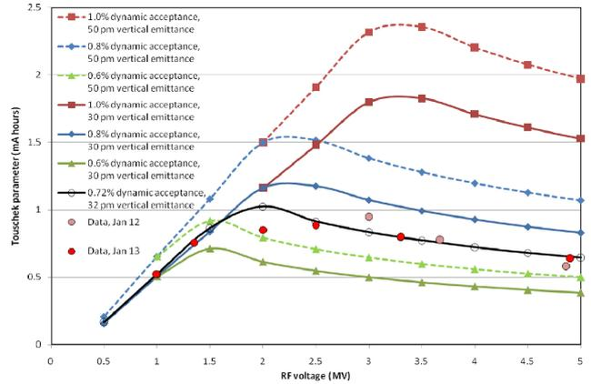
Figure 6: Data and simulation results for Touschek lifetime measurements in the CesrTA low emittance lattice at 2.085 GeV. The best match between the simulation and experimental data is the curve corresponding to 32 pm vertical emittance with a dynamic acceptance of 0.72%. The measured acceptance was 0.8%.
