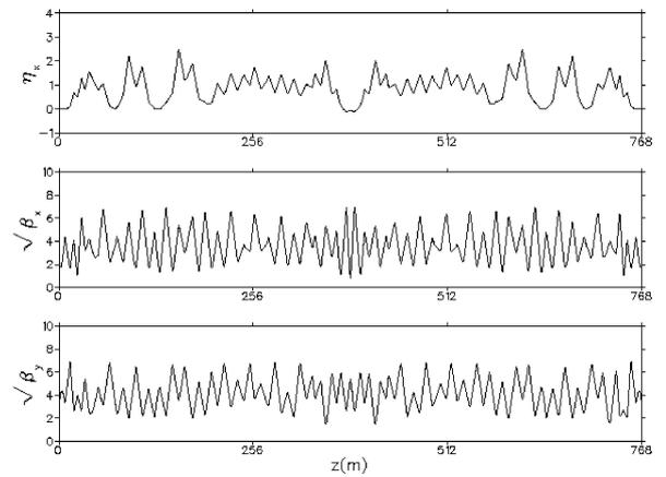
Figure 2: Lattice functions for the CEsrTA 2.085GeV baseline lattice.
