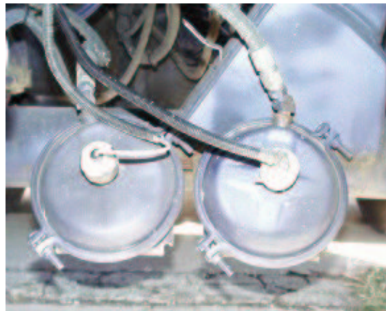
Figure 20: Brake Actuator: Air Pressure Transducer
