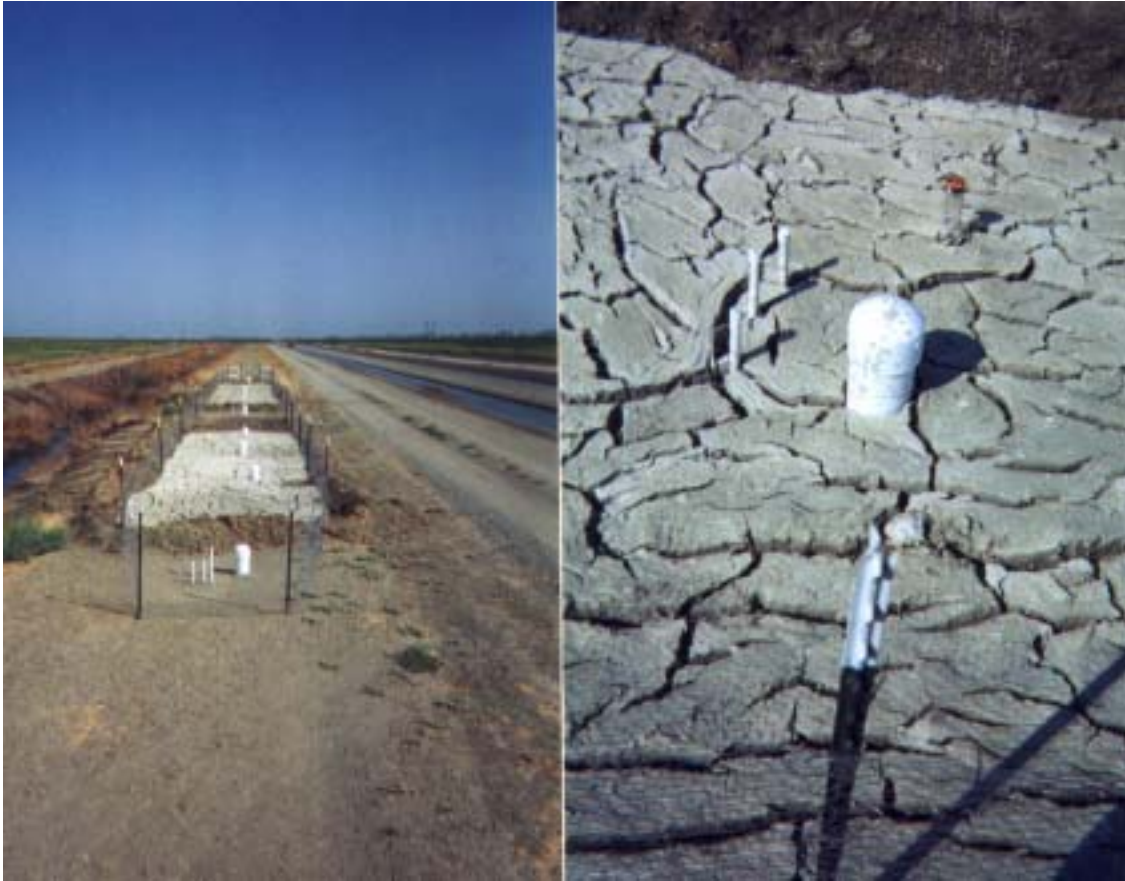
Figure C.7. Left: Sites EP-2 and EP3 after a few days of drying (9/9/99). Close-up view of drying cracks around one of the monitoring clusters (right).
