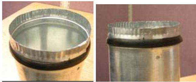
Figure 1. Inner PEGIT duct fitting showing rubber seal
