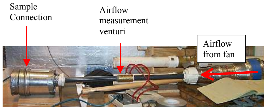
Figure 4. Phase 2 test apparatus for leakage testing.
