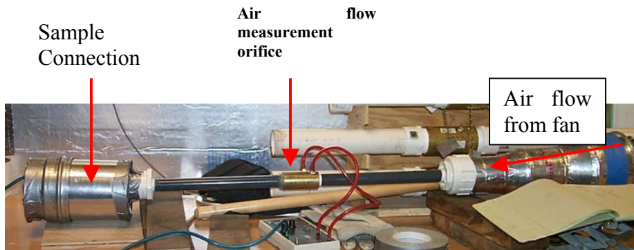
Figure 3. Test apparatus for leakage testing.
