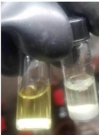
Image 1.1. Left – Difference in observed color of reaction where B 2 (OH) 4 is omitted (left) and included (right). A clear yellow color is observed when B 2 (OH) 4 is omitted, indicating no reaction is occurring.
