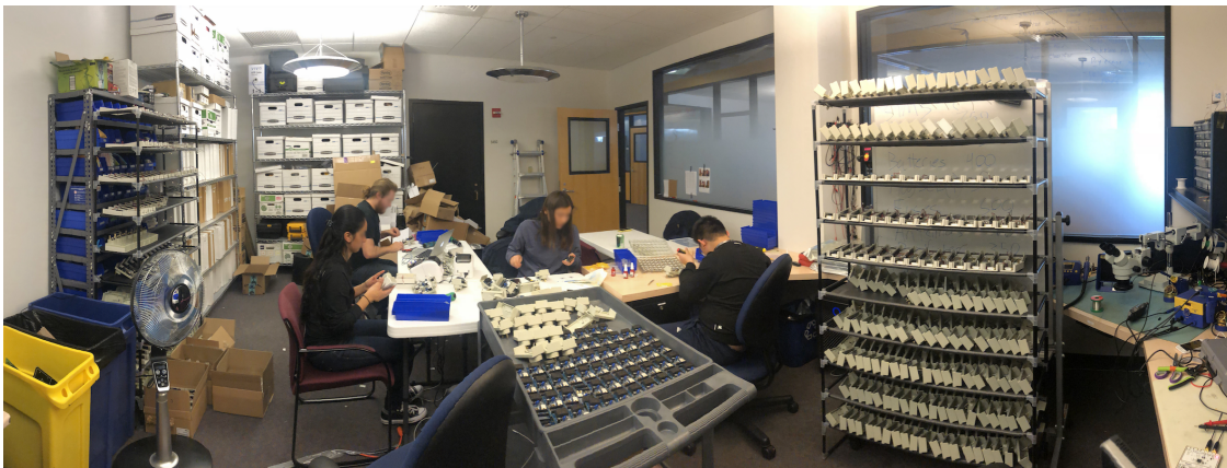
Figure 6.2: The PowerWatch assembly line. Over the course of four weeks, 10 undergraduates worked 110 person-hours to assemble 295 PowerWatch sensors. They were responsible for assembling the plug; screwing together the enclosure; attaching the circuit board; connecting the battery, antenna, SIM card and SD card; and provisioning the device with base firmware. They worked from team-created assembly manuals and training materials.
