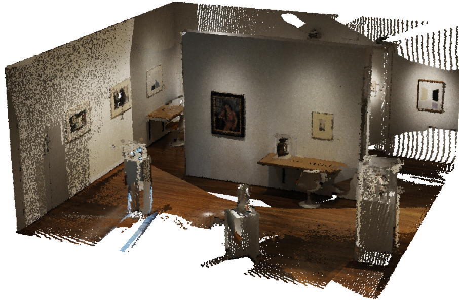
Figure 6.13: This thoroughly scanned partition wall may have a higher point count than the partially scanned boundary wall in the background. Note that this point cloud shows a different room from the sample data used in this study.
