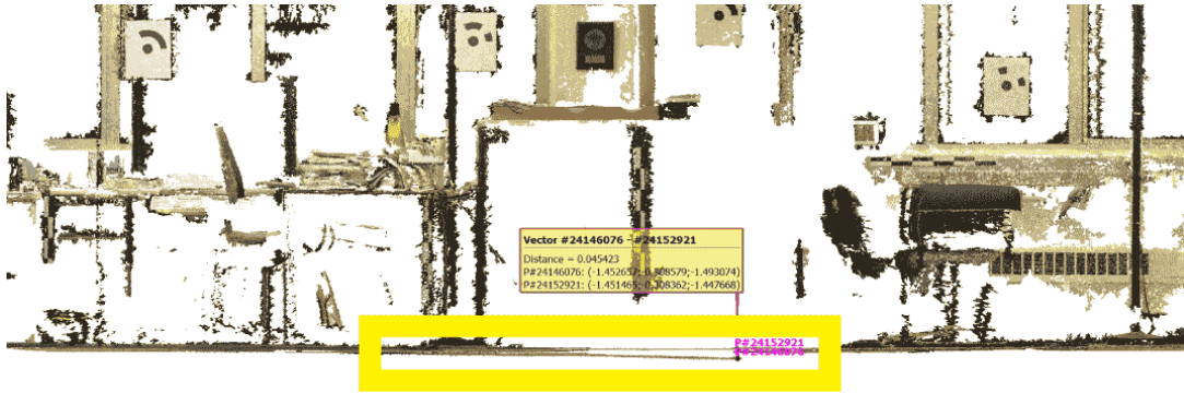
Figure 4.24: Side view of office point cloud from D3100 photos. Note the 4.5 cm vertical gap in the floor.
