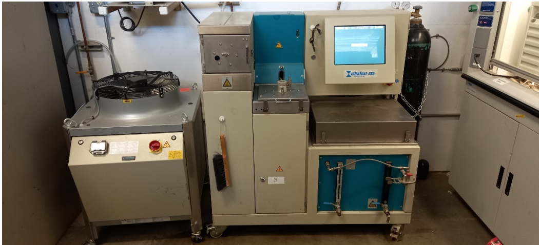
Figure 2.6: Closed-loop binder extraction system.
