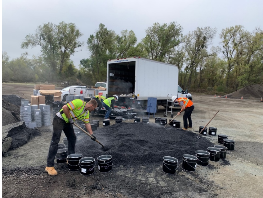
Figure 2.4: Sampling from hot drop put in buckets and boxes for QA sampling (each person is sampling from a quadrant of the pile of hot mix).
