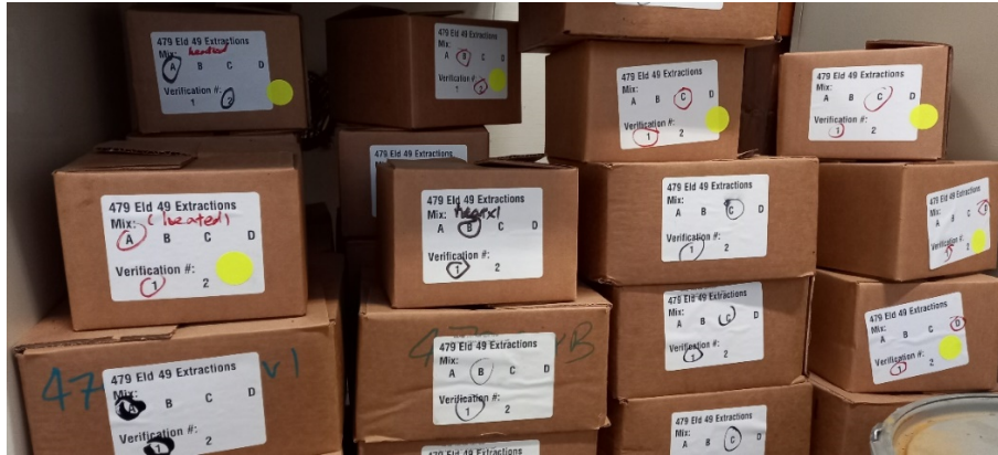
Figure 2.5: Loose plant mix samples stored in cardboard boxes in temperature-controlled environment before extraction.
