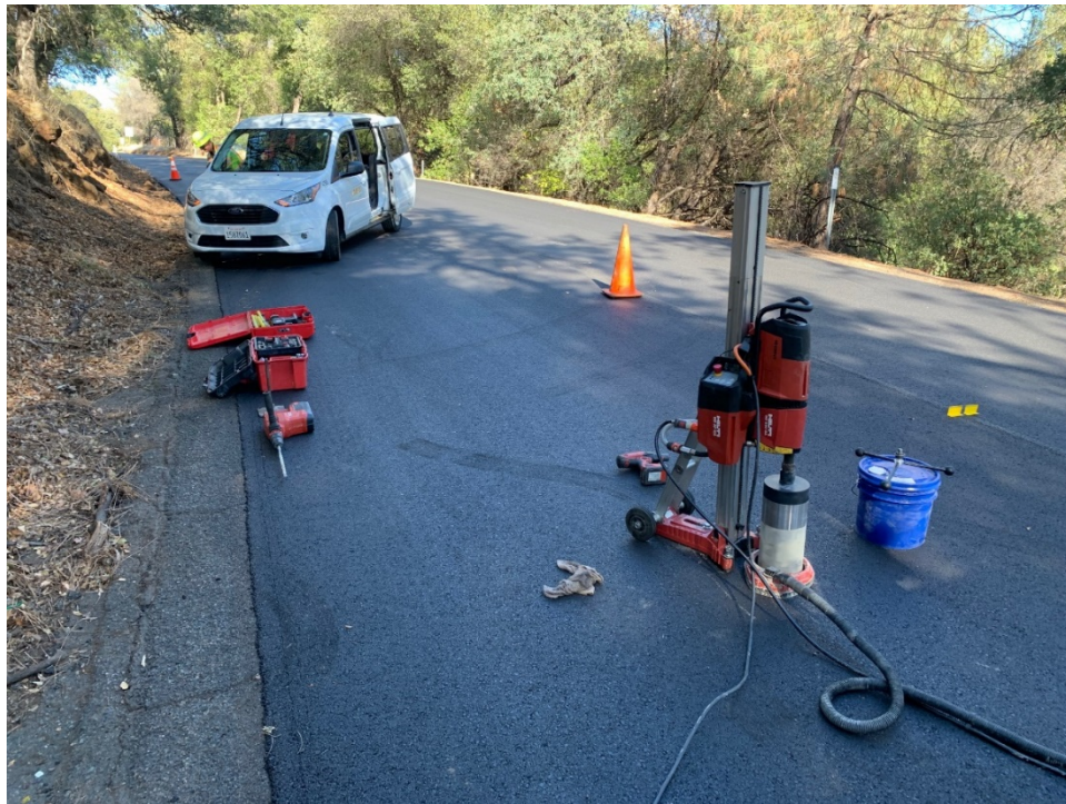
Figure 5.11: Sampling cores from new pavement.
