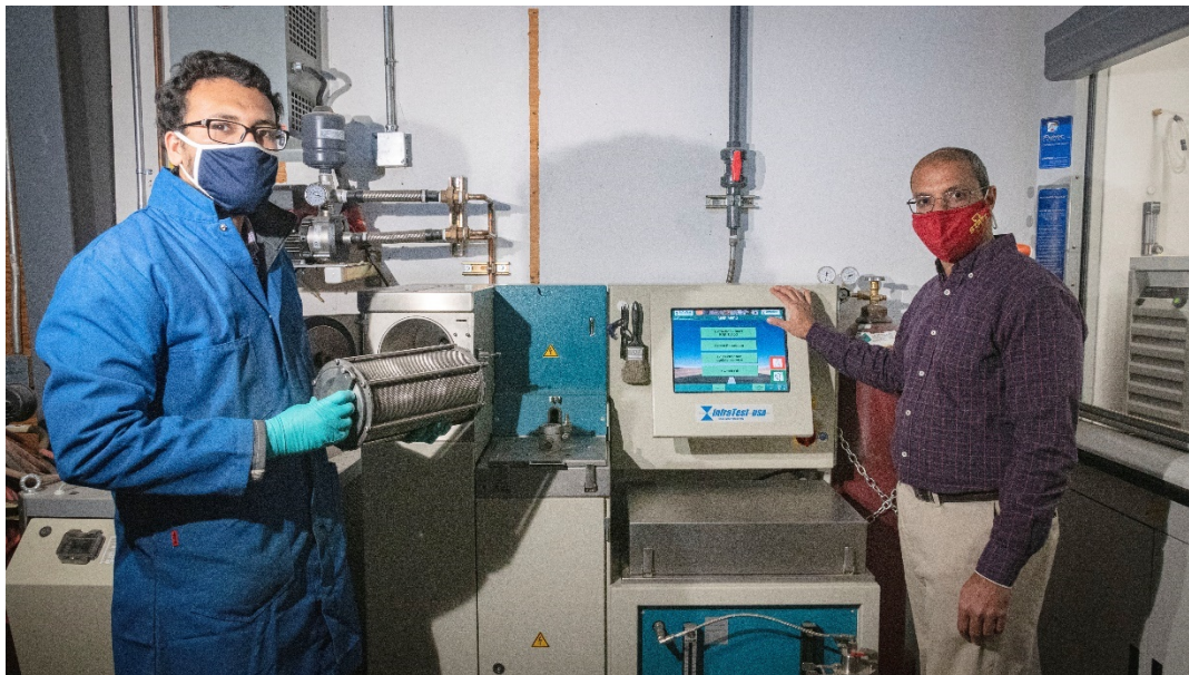
Figure 2.7: Placing extraction cylinder with sample into extraction system.
