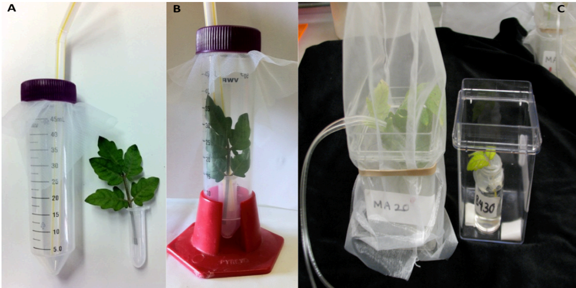
Figure 3.1A-C: Tomato detached leaf assay experimental set up. A-B) Detached tomato leaf placed in microfuge tube and 50ml tube with a straw to add water C) Detached tomato leaf in vials attached with a tube placed in magenta box.
