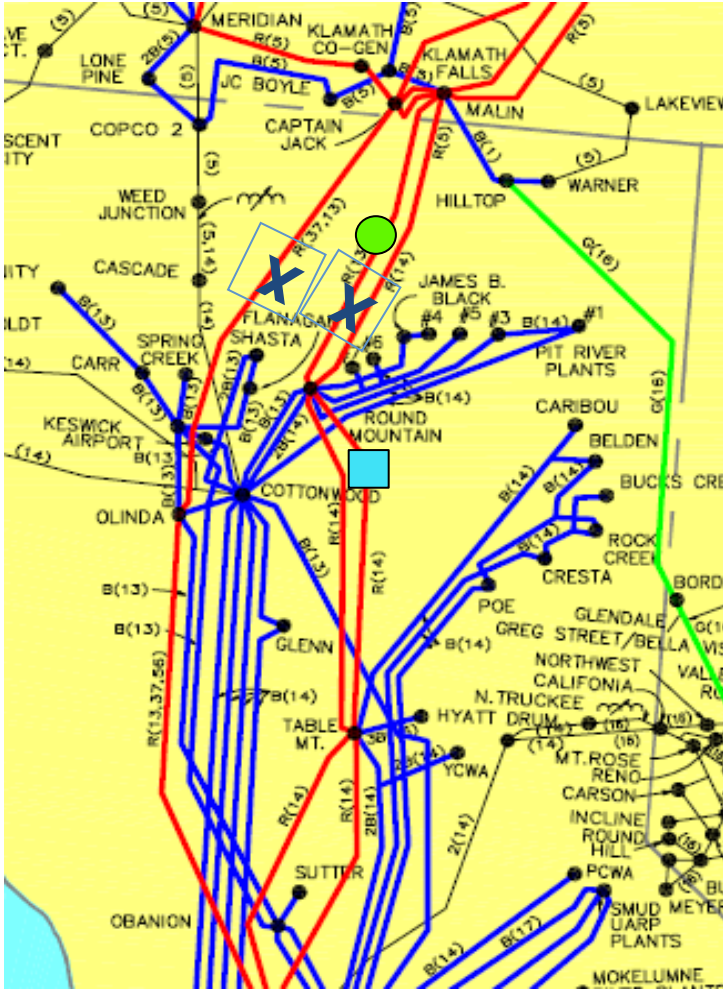
Figure 68. Relay at Malin, Monitoring Malin – Round Mt. #1 Line
