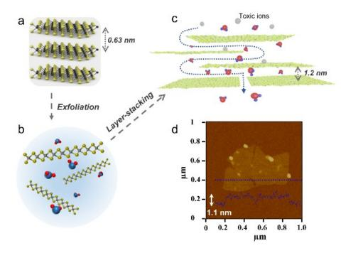
**Figure 1.** Schematic illustration of exfoliating bulk  $MoS_2$  materials (a) to create an aqueous suspension of  $MoS_2$  monolayer nanosheets (b) and reassembling the nanosheets into a layer-stacked  $MoS_2$  membrane (c) for adsorptive filtration targeting the removal of toxic ions. (d) The AFM image of a monolayer  $MoS_2$  nanosheet with a depth profile revealing a thickness of  $\sim 1.1$  nm.
