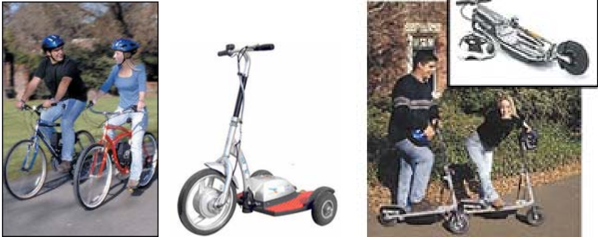
Figure 2.2. a) electric bicycle; b) electric 3-wheel scooter; and c) electric 2-wheel scooter.
