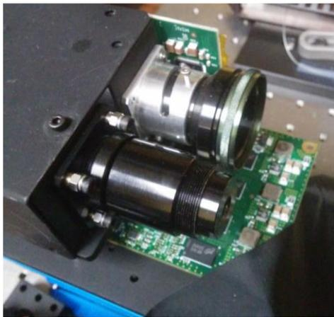
Figure 25. CEL-5500 DMD projector used to spatially modulate the light source into structured-light patterns.
