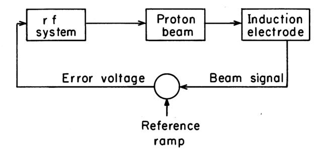
Fig. 2. Feedback loop for electronic beam spiller.
