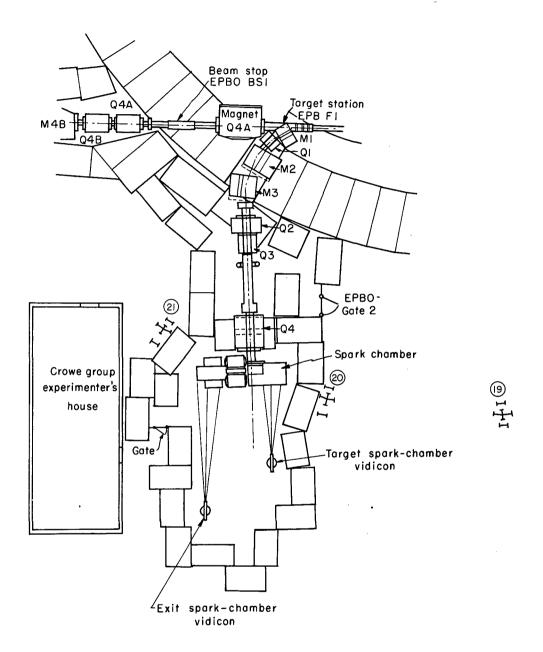
Fig. 6. EPB F<sub>1</sub> target station and beam transport for Crowe group's experiment.
