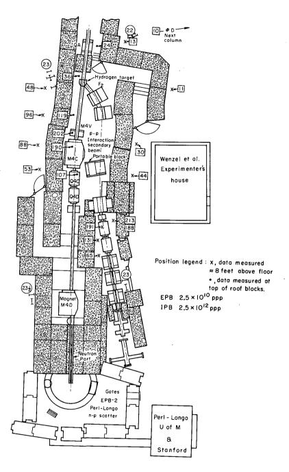
Fig. 5. Phase II external proton beam transport shielding modified to accommodate the Lofgren group p-p scatter work. (Fast neutron flux values are enclosed in squares; the values marked with an x were determined at roughly 8 ft. above floor level, and those marked with o were determined at roof level.) Column numbers are enclosed in circles.
