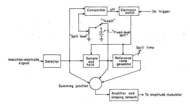
Fig. 3. Block diagram of electronic beam spiller.
