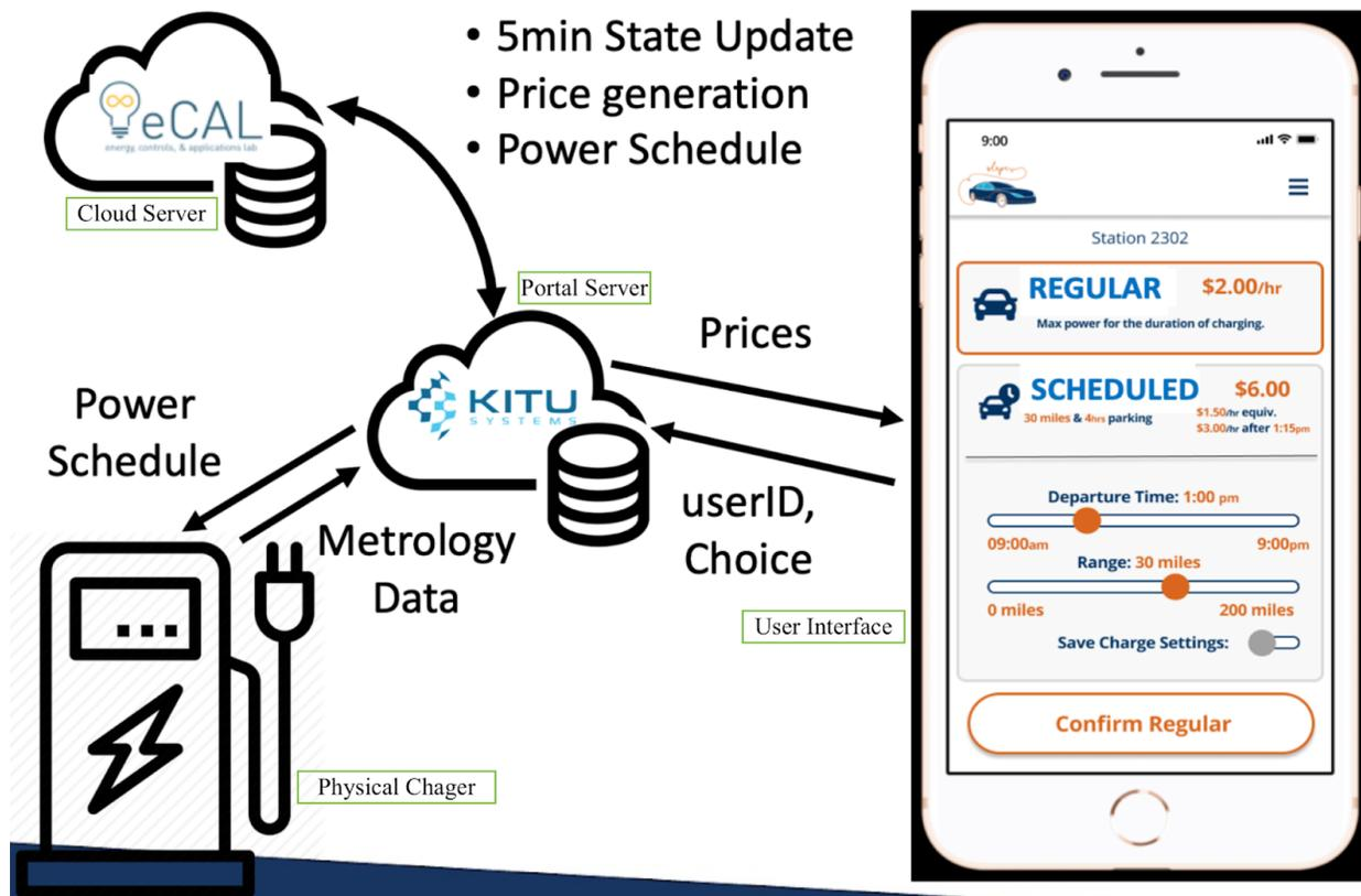
Figure IV-1: Schematic of the SlrpEV ecosystem
