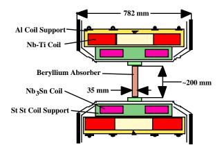
Figure 2. A Cross-section of the MICE Focusing Magnet with a Nb<sub>3</sub>Sn Insert Coil and a Beryllium Absorber
