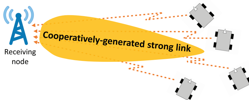
Figure 1.1: Distributed robotic transmit beamforming. The robots can cooperatively generate a strong communication link by optimizing their locations.
