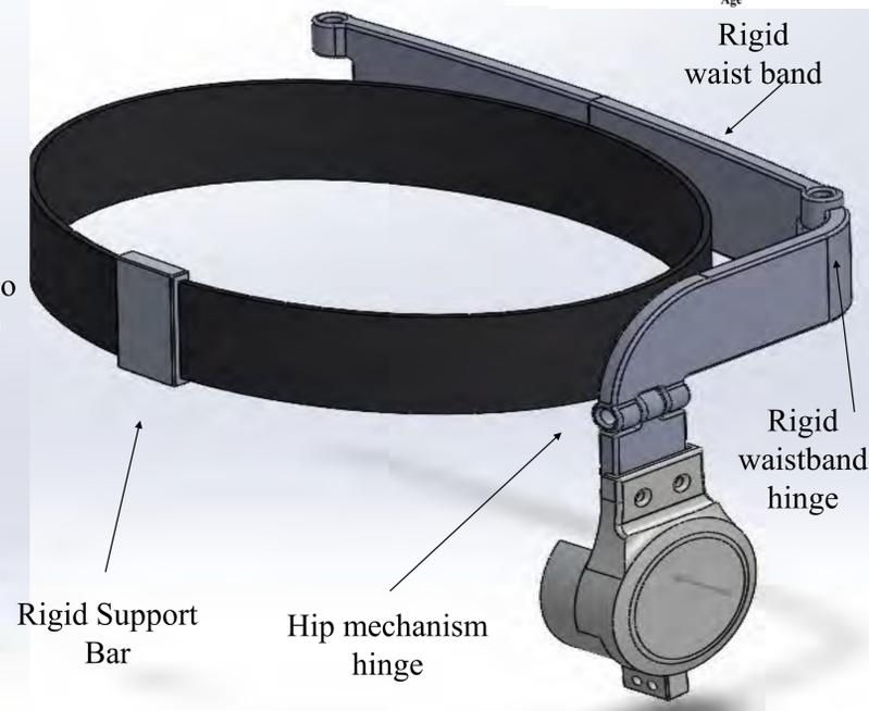
CAD of Hip Mechanism
