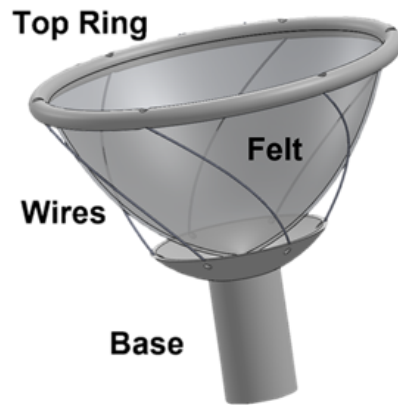
Figure 2.10: Drawing of primary components of the prototype
