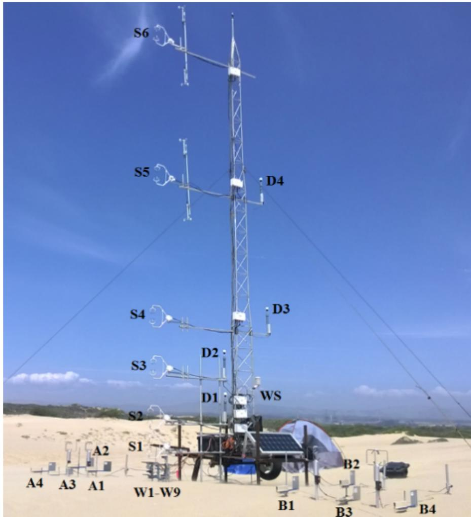
**Figure 2.1:** The experimental setup at Oceano Dunes. Instrumentation includes six sonic anemometers (S1–S6), nine Wenglor particle counters (W1–W9), eight Big Spring Number Eight sand samplers (A1–A4, B1–B4), four optical particle counters (D1–D4), and a weather station with temperature and humidity sensors (WS) (following *Martin and Kok* (2017)).
