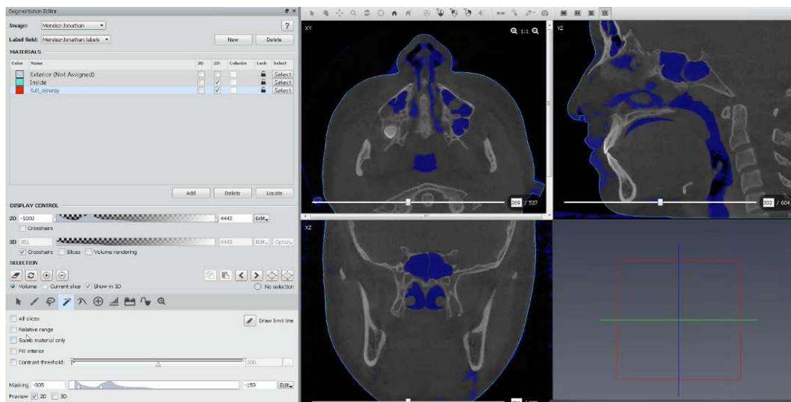
Figure 4: Amira automated segmentation selectively includes the airway as the area of interest
