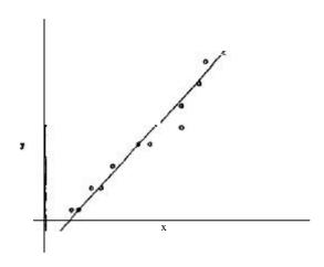
Model<sub>D</sub>:  $y_i = a + bx_i + e_i$ , where the ei have a N(0,  $\sigma^2$ ) distribution. Validation: Compute the least squares estimates for a and b and determine if the residuals,  $e_i$  have a N(0,  $\sigma^2$ ) distribution.
