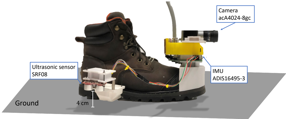
Figure 4.7: The Lab-On-Shoe platform integrated with a downward-facing ultrasonic sensor. The camera in the picture was not used in this work.
