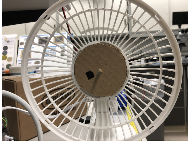
Figure A.31: The FOV of the DVS128 represented in a conventional camera in the rotated dotted plate experiment.
