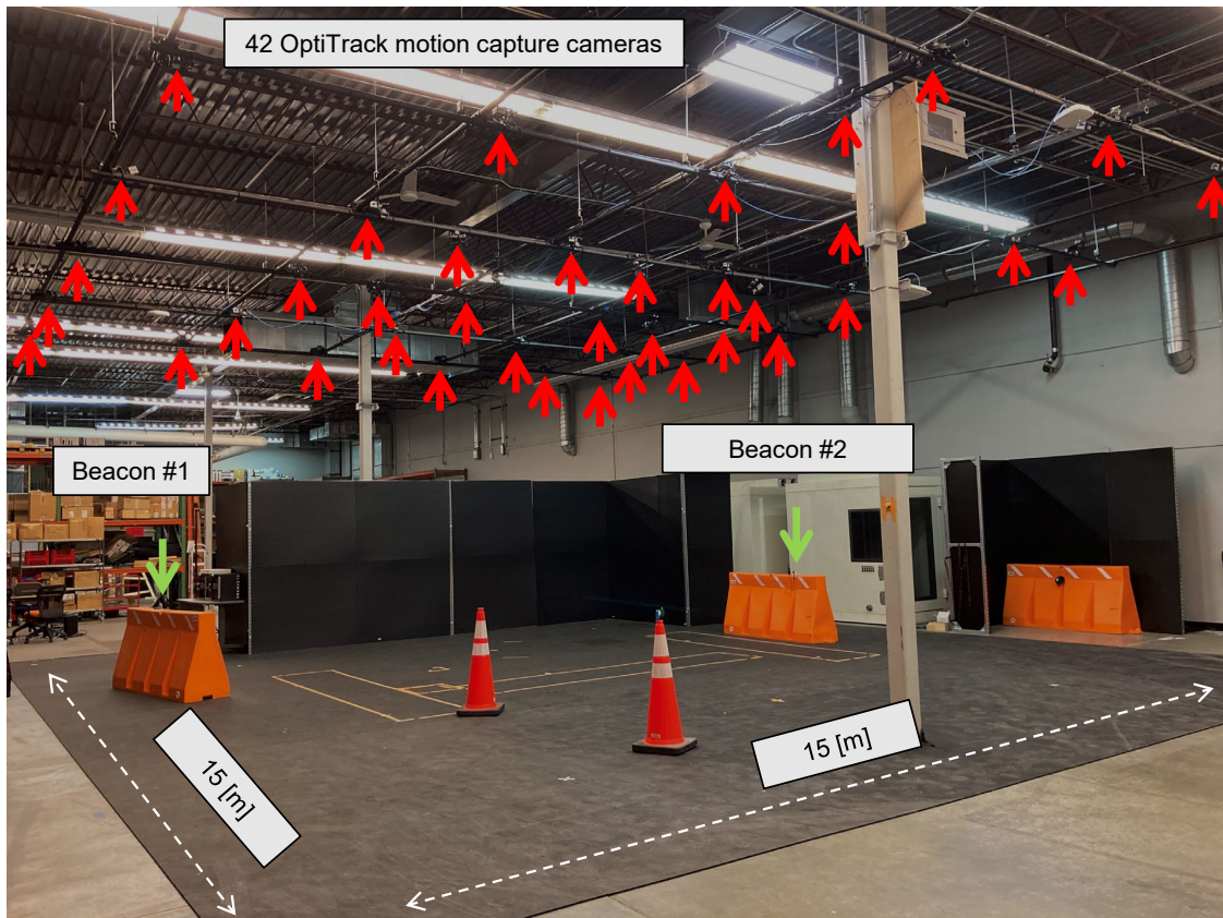
Figure 9.15: Experimental scenario for the experiment discussed in Section 9.3.3. 42 OptiTrack motion capture cameras were mounted on the ceiling of a warehouse and obtain the ground truth position and orientation. Two beacons were placed on top of the orange barricades during the experiment. The operation range of the motion capture camera system was around 15 [m] \times 15 [m].
