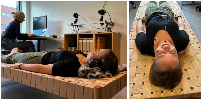
Figure 1: Physical movement was monitored with Qualisys motion capture using eight sensors on feet, hands, cheeks, abdomen and chin.
