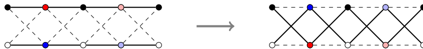
Figure 4.4: Two representations of the same network. Interchanging the positions of relay nodes in every other hop changes the representation of the network from a weak interference setting to a strong interference setting. This works only when the number of hops, L , is even.
