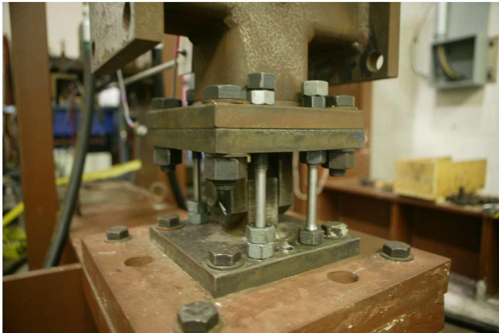
Figure 3.13: 1-DOF \mu -NEES experimental setup clevis and coupon configuration. Total of 4 steel coupons are used, two on each side.
