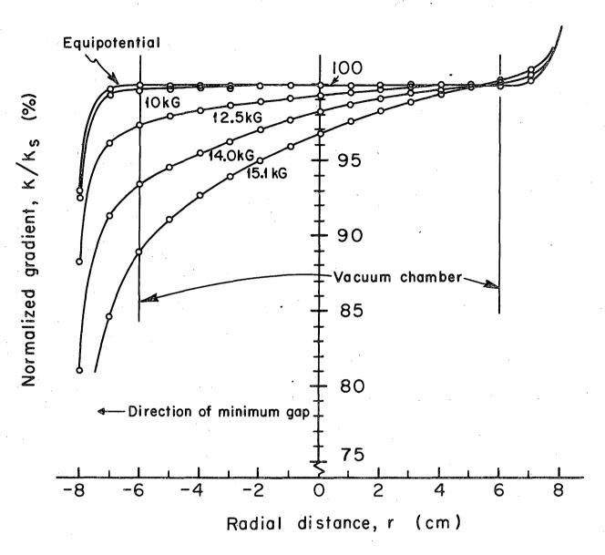
Fig. 2. Computed gradients, 200-BeV gradient magnet.
