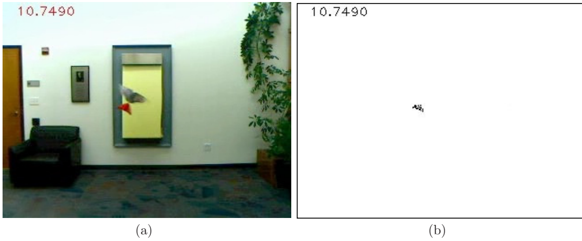
Figure 4.5: A camera captured image of a free flying ornithopter (a) and the orange blob of the ornithopter found by the blob detection algorithm (b).
