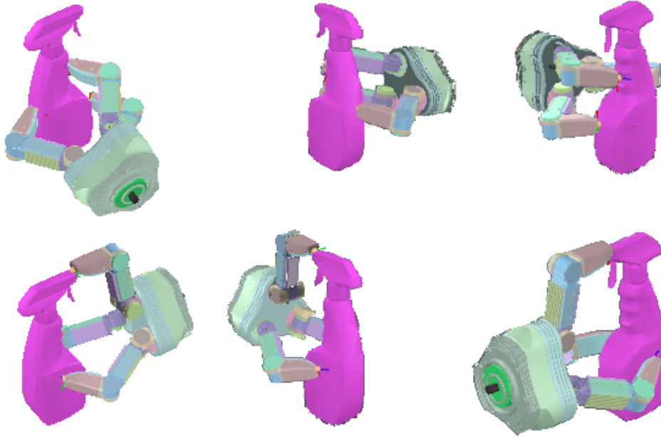
Figure 10: Top figures: best grasp determined using the grasp wrench space quality measure. Bottom figure: best grasp determined using the object wrench space quality measure. Each grasp is shown from three different view points to outline the differences.
