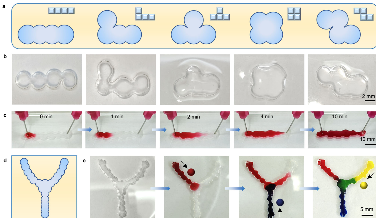
Fig. 6 | Complex patterns of droplet networks. a, b Schematics and optical images showing Tetris composed of droplet networks. c Optical images showing the transmission of a dye solution within the linear droplet network channel; [\text{Amaranth}] = 1.0 \text{ mg mL}^{-1} . d Schematic showing the “Y” type of droplet network
