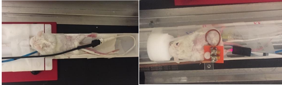
Figure 2.14: Mouse monitoring setup. Mouse is placed prone on a pressure pad (blue line) to monitor respiration. The black and white cable monitors animal temperature. On the right, a sensor is placed on the mouse paw to monitor blood oxygenation. The surface coil is tightly screwed right above the tumor to obtain optimal signal.
