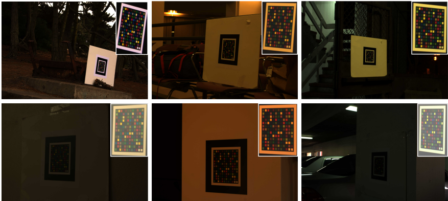
Fig. 3. Examples of images with the “test” color checkerboard, used in our experimental tests. The inset at each picture shows the brightness-rescaled, zoomed-in checkerboard detail.
