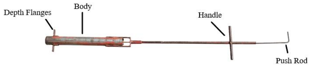
Photo 2.1: Soil core sampling device constructed by the author
