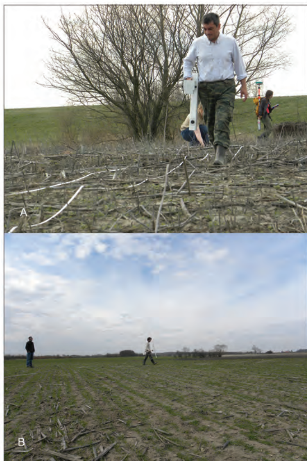
Figure 6.1. Magnetic survey by Apostolos Sarris using the Bartington G601 fluxgate gradiometer (A). Magnetic survey by Nikos Papadopoulos using the Geoscan FM36/256 fluxgate gradiometer (B). Figure by William A. Parkinson.
