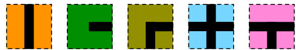
Figure 4: Set of tiles for modeling microfluidic devices with regularly spaced, orthogonally intersecting straight channels. Dark regions denote the fluid pathways. The tiles are shown in top-view.
