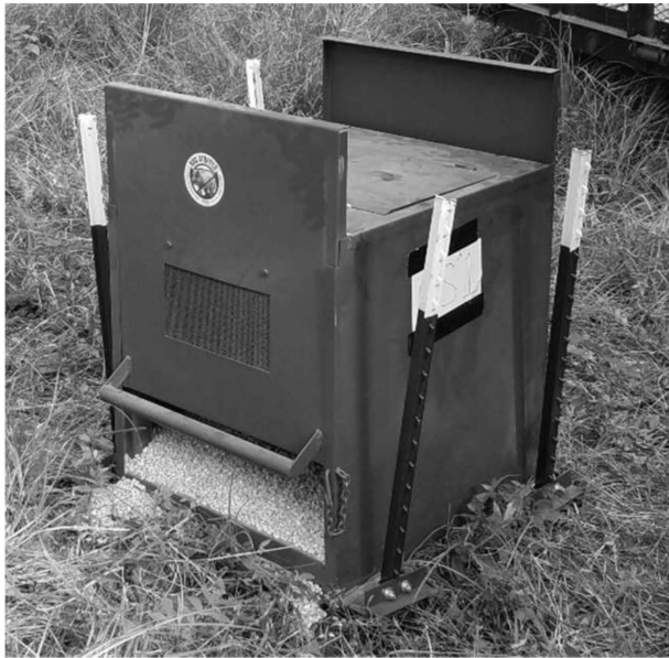
Figure 1. Comparison of Hog Stopper™ feeder with 7.7 kg guillotine doors (left photo) and Brower® commercial feeders with 4.5-kg steel bars attached to doors (right photo).
