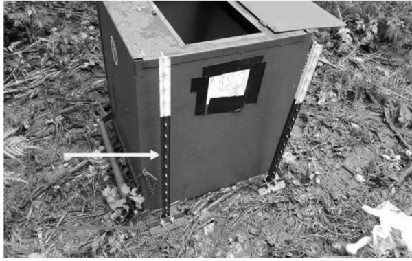
Figure 2. All Hog Stopper™ feeders are secured to the ground with v-bolts and studded t-posts which keep non-targets from tipping them over.
