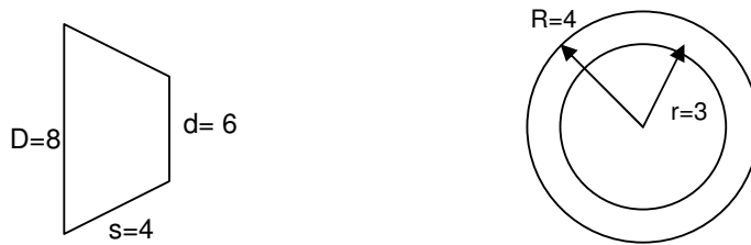
Fig. 9 Projected surface area estimation for two different orientations of a conical spiral chip
