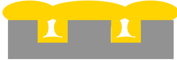
Figure 3. Voids left after electroplating the sputtered seed layer.
