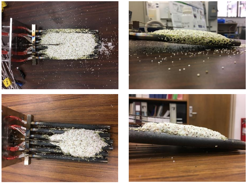
Figure 5.11 Aggressive pebbles sintering into solid blocks at the creep region extending up to 1 cm away from the heaters
